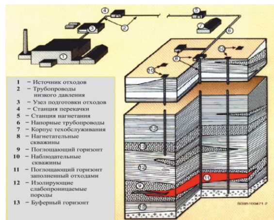
Figure 2. An indicative plan of liquid nuclear waste disposal; (1) A waste generator, (2) Low pressure pipeline, (3) A waste processing unit, (4) Relif station, (5) Injection station, (6) Force mains, (7) Maintenance building, (8) Injection wells, (9) An absorbing layer, (10) Observation wells, (11) A waste-holding layer filled with waste, (12) Isolating impenetrable (waterproof) layers, (13) A buffer layer
