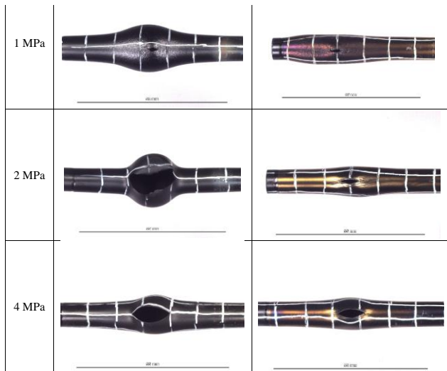
Figure 6. Visual analysis of Cr cold spray coated Opt. ZIRLO™ after high-temperature creep test and bursts. Reduction of deformation of the coated samples is clearly visible.
