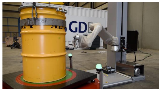
Figure 7. Drumcar©, radioactive drum characterizer
