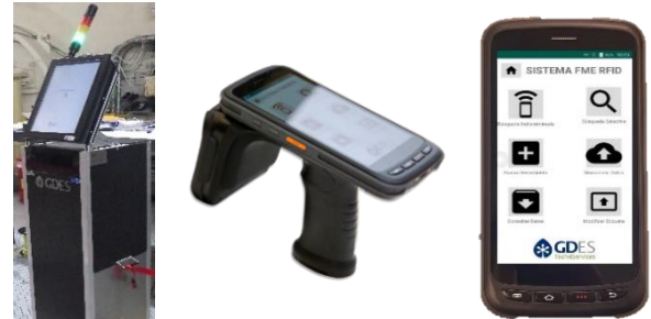
Figure 3. Components. Mobile beacons and portable reader.
