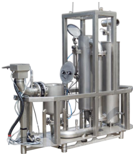
Figure 2. Filtrabris©, aspiration and filtration system for the analysis of debris accumulated in spent fuel elements
