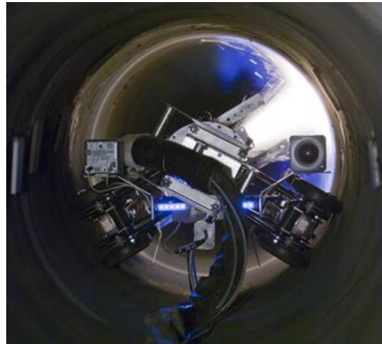
Figure 6. Tirant©, robot for the arc-spray metallization of large bore pipes
