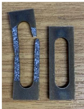
Figure 6. Failed vs new S2BT specimen.
