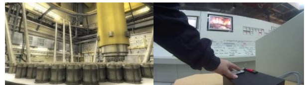
Figure 11. Digital twin of refueling engine embedded on simulator control room developed by Tecnatom
