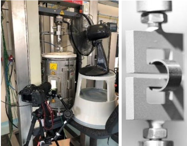
Figure 2. Photograph of the assembly on a tensile test machine (left) and of a C-Ring into the swings (right)
