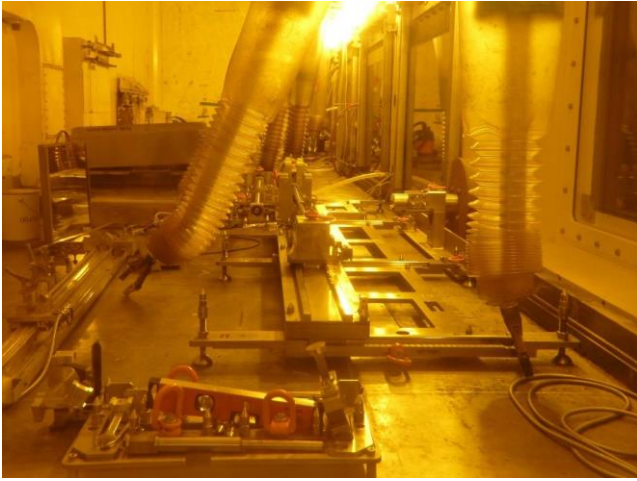
Figure 13: Gamma spectroscopy rig installed in a hot cell.
