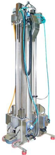
Figure 5. LD4+©, robot for mechanical cleaning of reactor vessel bolt housings
