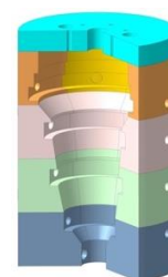
Figure 2. Melter pool made of refractory ceramic blocks.
