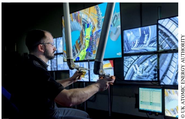
Figure 2. JET Remote Handling Control Room and MASCOT vision system.
