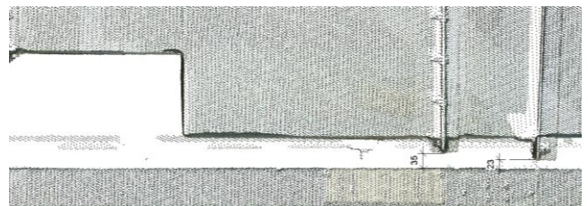
Figure 4. Point cloud of the detail of the distance between cable tray and HVAC. Almaraz I NPP (Spain)
